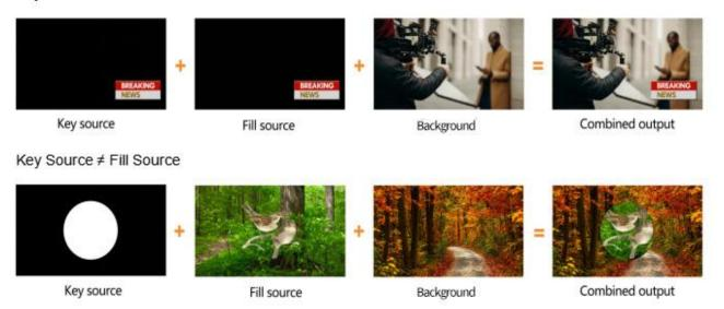
Switching a video with background to PVW window, and turn on the Luma Key. Press the menu knob to enter the setting interface. Under Luma Key sub-menu, user can assign the fill and key source from various options including Black/ Color Bar/ Color1/ Color 2/ IN1/ IN2/ IN3/ IN4/ Image (import from USB disk). Configure and adjust the Key parameters including Clip/Gain/mask to achieve the effect needed.
