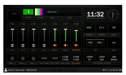
The information of user name, working time, CPU working temperature, system time keeps displaying in the bottom of the Status/Menu page.
